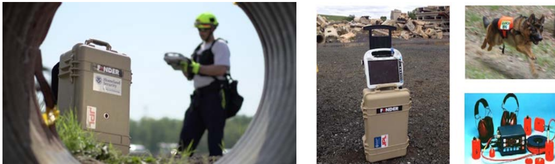
FINDER's microwave radar complements search dogs and sound tools to detect the heartbeats of victims from up to 100 feet away.
